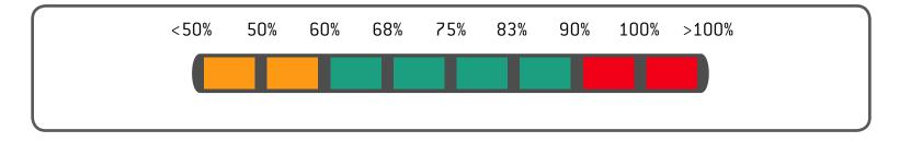
The first two LEDs, coloured orange, signal a heart rate less than 60% of the theoretical maximum heart rate; the four central LEDs, coloured green, signal values between 60% and 90%; the two red LEDs signal a heart rate greater than 90%.
