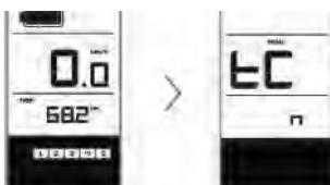
**Adjustable parameters:** Erasing the data such as TRIP, MAXS, AVG, tC. Setting unit km/mil (S7). Adjusting the automatic display backlight (bL0), display brightness (bLI). Setting the display automatic switch off function (OFF). Maintenance warning (nnA).
