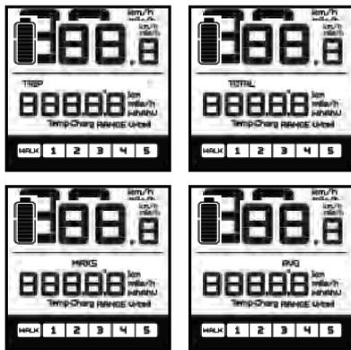
**Battery charge status indicator:** Battery charge level (displays 10 degrees at maximum charge; 1 degree = 10% capacity). If discharge occurs, the battery contour will flash. The battery must be charged immediately.
