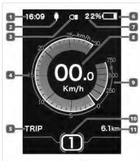
**1. Time:** The time is displayed in a 24-hour format and shows the current time.
