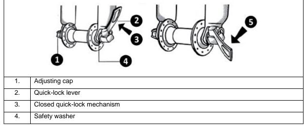
5. Open quick-lock mechanism
