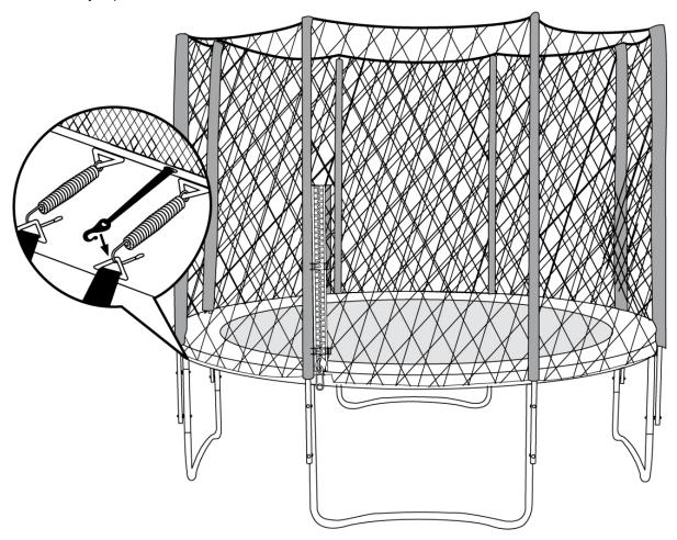
**STEP 5:** Close the zip on the safety net (7) and hook it to both security fasteners.
