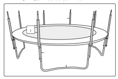
**STEP 2:** Spread the safety net (7) on the trampoline's jumping mat. Make sure the pockets meant to hold the upper pole A face upwards. Align the pockets with the upper pole A.
