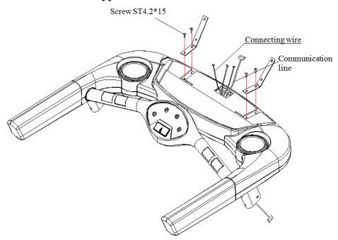
Set meter stator on upper cover of meter. Use 4 pcs of Screw ST4.2\*15 to solid meter stator. (Fasten screws).
