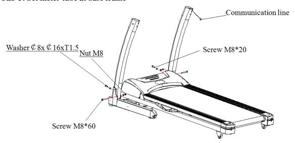
Set meter tube at base frame, use 2 pcs of Screw M8\*20 and 2 pcs of washer, 2 pcs of Screw M8\*60, 2 pcs of washer and 2 pcs of nut to solid the meter tube (Don't fasten screw at first)
