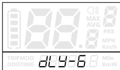
Delay Time of Battery Power Interface
