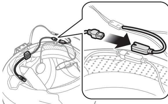
**Note:** The shortest cable is for the microphone.
