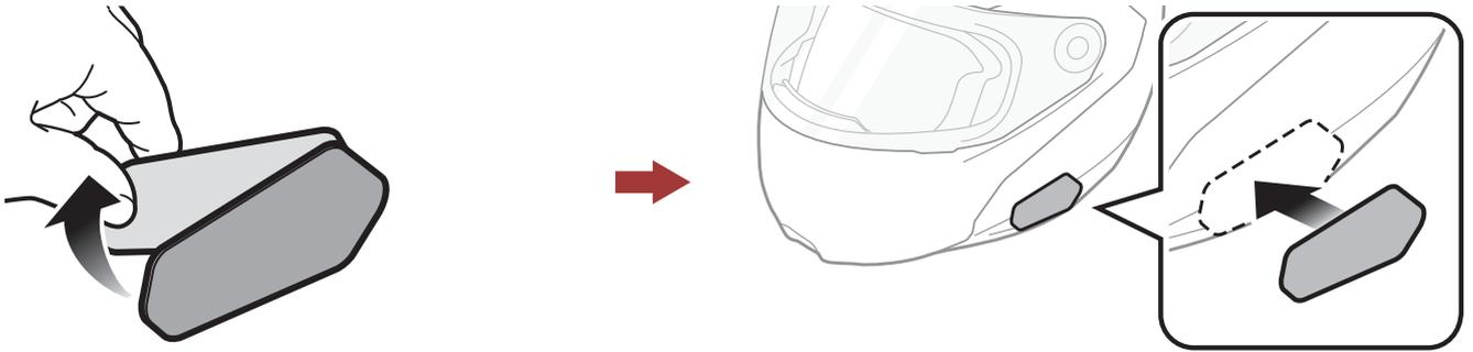
3. Peel off the cover of the adhesive tape of the hook fastener for main unit and attach it to the back plate of the main unit.
