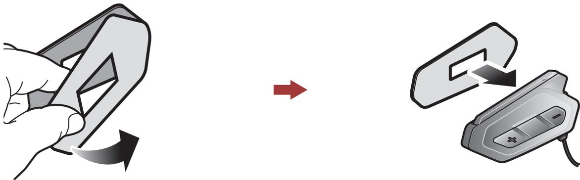
4. Attach the main unit using the hook and loop fasteners that you fitted. Make sure that the main unit is firmly attached to the helmet.
