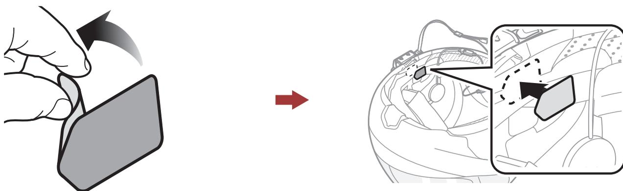
2. Attach the wired boom microphone's mounting plate to the hook and loop fastener.
