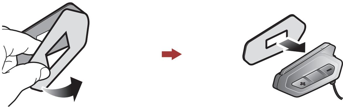
3. Peel off the cover from the other side of the double sided adhesive tapes and attach the main unit on the left side of your helmet.
