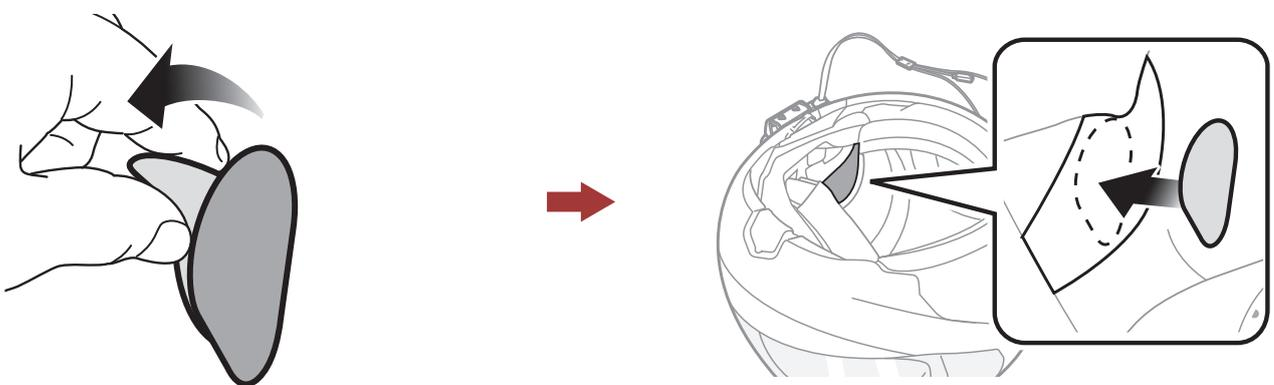
2. Attach the speakers to the hook and loop fasteners for speakers inside the helmet.
