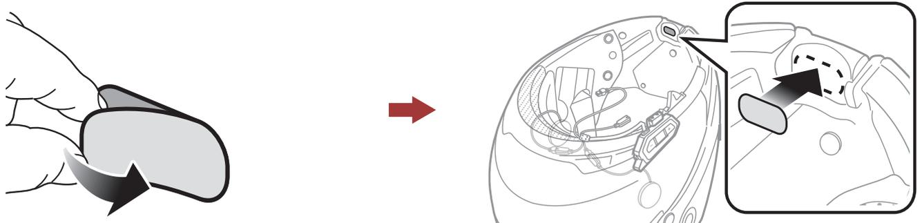
2. Attach the wired microphone to the hook and loop fastener for wired microphone.
