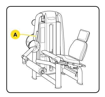
Pay particular attention to the parts of the equipment with labels indicating "BEWARE OF CRUSHING".
