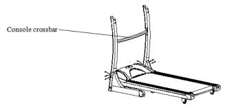
Assemble the console crossbar (60) to the console masts (51, 58) with four M8x20mm bolts (59) and washers (56). (Do not tighten the bolts)
