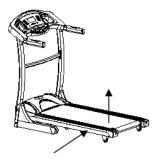
NOTE: Make sure that the locking bolt is locked in place correctly.
