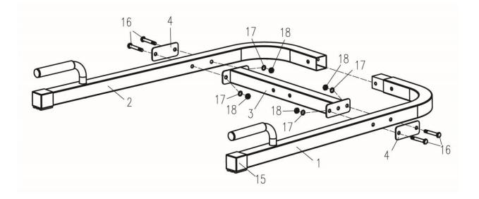
Connect Left Lower Baseframe (1) to Right Lower Baseframe (2) using Lower Cross Bar Support (3) and secure with 4 Bolts (16), 2 Metal Support Plates( 4), 4 Washers (17) and 4 Nuts (18). Place End Caps (15) on ends of Baseframe 1 & 2.
