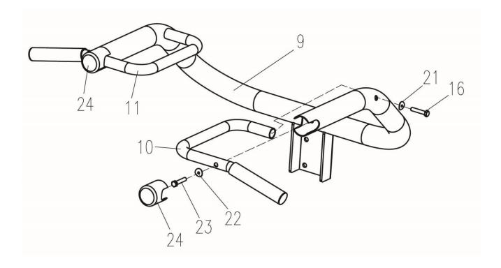
Connect Handlebars (10 &11) to Upper Pull Up Frame Assembly (9) using Bolts (16) and Washers (21). Connect Handlebars to Upper Frame Assembly using Screws (23) and washers (22). Place Round Caps (24) over End of Handle Assembly.
