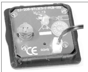
Open the Computer (Part: 22). Install the battery into the correct position.
