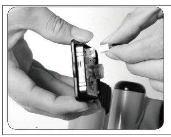
Connect the Computer (Part: 22) with Main Frame cable (Part: 1).
