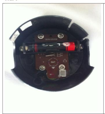
Open the Computer (Part: 22). Install the battery into the correct position.
