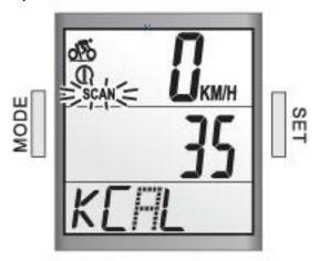
When in Kcal mode, press "MODE" key shortly, then the icon of scan will appear that cycle computer will automatically scan your current active result in different mode from CLK, TM, MXS, AVS, DST, ODO, to KCAL. It will automatically switch from one mode to another one every 4 seconds.
