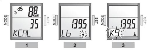
Go KCAL MODE by pressing "MODE" key, then press "SET" key for 3 secs to go User Set. By pressing "SET" key & "MODE" key alternatively to enter the correct personal data. Press "MODE" key for 3 secs when complete.
