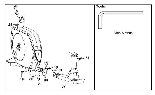
Remove two M8x30mm Bolts (85), four M8x15mm Bolts (18), and six Ø16xØ8x1.5t Washers (53) from the Rear Main Frame (67). Remove bolts with the S6 Allen Wrench provided.
