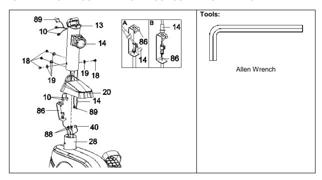
Remove four M8x15mm Bolts (18) and four Ø8 Curve Washers (19) from the Front Main Frame (28). Remove bolts and curve washers with the S6 Allen Wrench provided.
