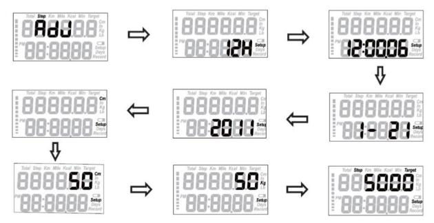
Press MODE to enter STEP mode. Press and hold the SET button for 2 seconds to enter SETUP mode as follows: 12-24 Hour Format / Seconds / Hours / Minutes / Month / Day / Year / Measurement Units / Stride / Weight / Target Steps.
