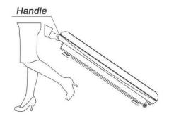
Two handles are designed on both ends of the middle cover. When moving the Product, lift the end opposite of the castor, grasp the handle and move the Product to the desired place.
