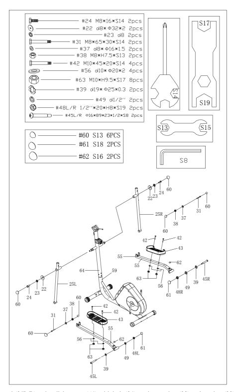
Secure swing rod (25L/R) to handlebar post (64) with bolt (24), spring washer (23) and washer (22); then attach end cap (60).
