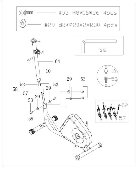
Connect tension control (52) with tension wire (57); and connect trunk wire 1 (10) with trunk wire 2 (58). Secure handlebar post (64) to main frame (59) with screw (53) and arc washer (29).
