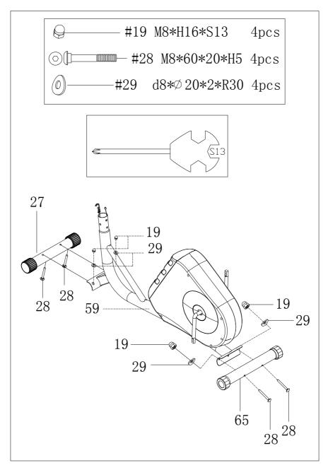
Secure front stabilizer (27) and rear stabilizer (65) to main frame (59) with bolt (28), arc washer (29) and nut (19).
