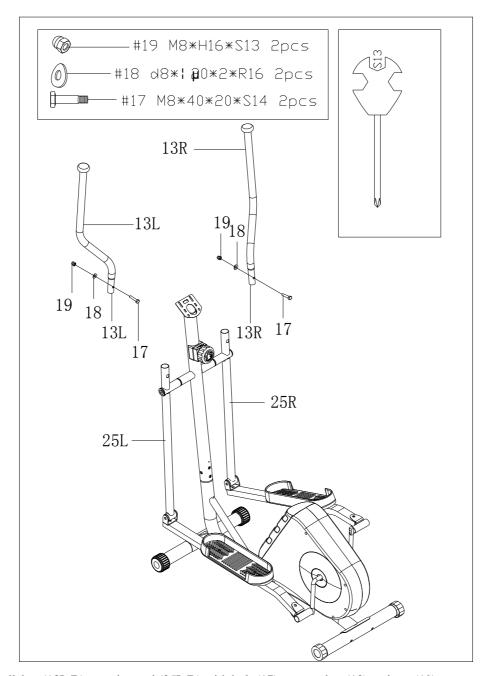
Secure handlebar (13L/R) to swing rod (25L/R) with bolt (17), arc washer (18) and nut (19).
