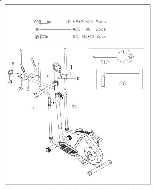
Secure middle handlebar (2) to handlebar post (64) with screw (8) and spring washer (23), then attach clamp cover (40).
