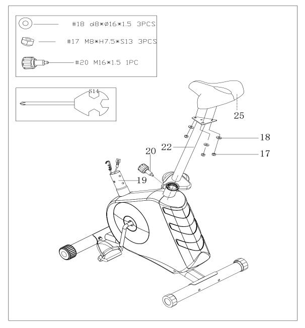
Secure the saddle (25) to the Seat post join (22) with the washer (18) and nylon nut (17)
