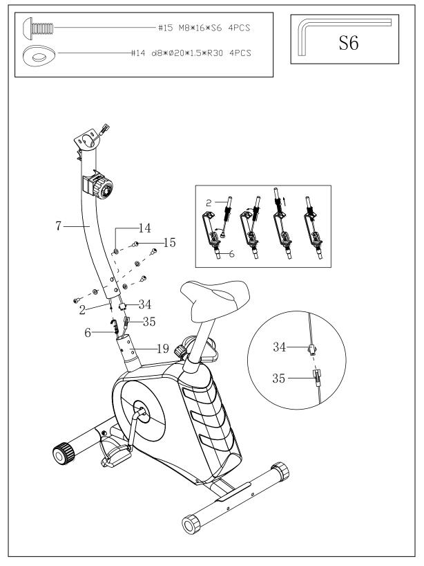
Connect sensor wire (35) with Trunk wire (34).
