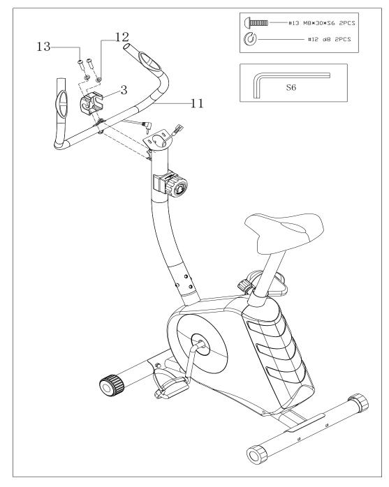
Fit handlebar join (11) into the cap of main frame tube join, lock with bolt (13) and spacer (12). Lock cap (3) into handlebar.
