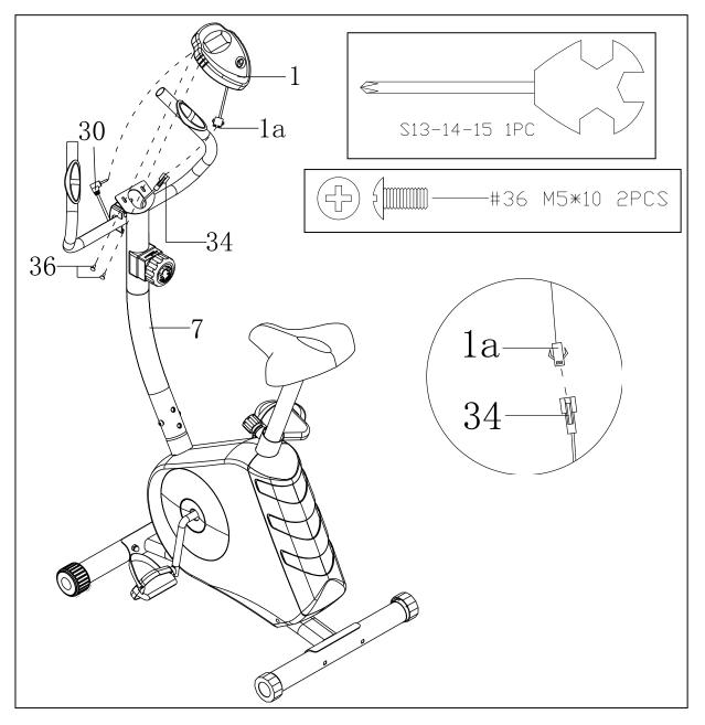
Connect computer wire (1a) with inductor wire (34). Lock computer (1) into computer board of force tube join (7) with bolt (36), insert wire (30) into the hold of computer's back.
