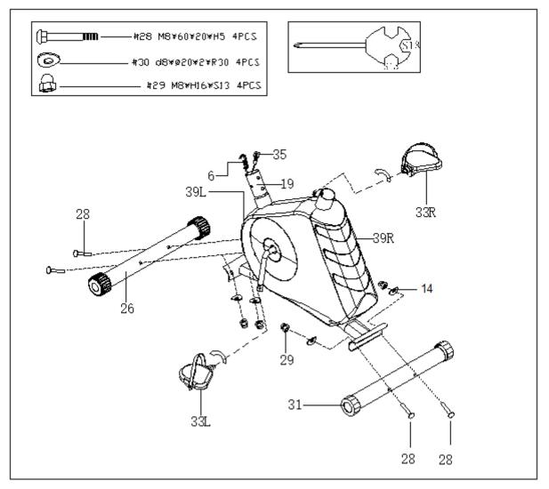
Attach front bottom tube (26), back bottom tube (31) to main frame join (19) with bolt (28), washer (14) and nut (29).
