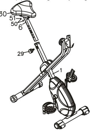
**NOTE:** DO NOT pull out the seat tube over the warning line "MAX" which showing on the tube. When you adjustable the height of seat.
