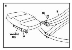
7. Move the Roller Carriage (6) to the position shown, and align the indicated hole in the Roller Carriage with the corresponding hole (not shown) in the Pivot Frame (3).
