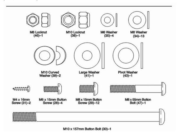
1. Attach a Base (2) to the Frame (1) with four M8 x 15mm Button Screws (29) and four M8 Washers (34).
