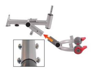
• Insert the front wheel into the frame (A).
