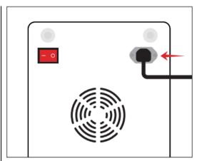
Plug the power cord into the device and then into the electrical outlet.
