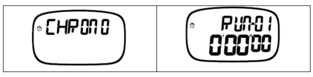
It measures and records lap times and split times up to 100 laps with Fastest lap alarm.
