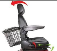
Use the levers to adjust the appropriate position of the seat and backrest.
