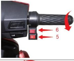
You switch gears with button 6, forward movement or reverse with button 5 (press the button to reverse) You control the speed with the gas on the right side
