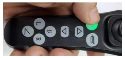
Press the reduce max. speed button on the wheelchair controller until the middle LED lights up.
