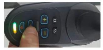
Press the reduce max. speed on the remote control until the power button stops flashing.
