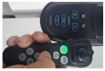
To change the angle of the backrest, press the B button, then use the arrows to adjust the angle.
