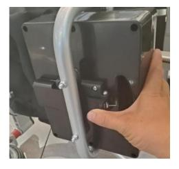
Grasp the battery and pull it out of the frame.
