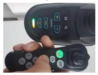
The LED on the wheelchair controller turns off and the controllers are paired.
