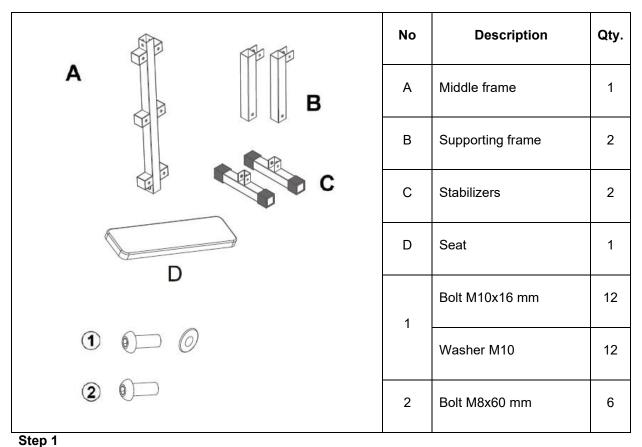
Join parts A, B and C using fastener #1: 12x M10 x 16mm bolts and 12 M10 washers.
