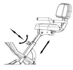
Pull out the frame angle adjustment pin and adjust the frame to the desired position. Then secure with a pin. There are 3 frame positions to choose from.
