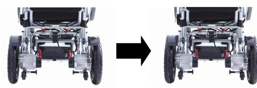
Push the armrests down and lock with the button by turning the button up.
