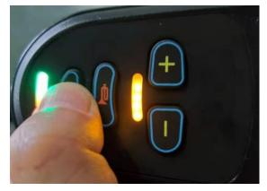
Hold down the down arrow on the remote control until the power button on the remote control stops flashing.
