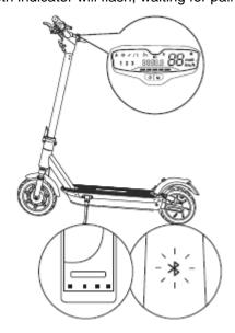
Use your smart device to pair the scooter. The Bluetooth icon stops flashing and lights up.
