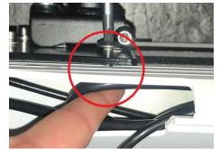
4. Reattach the side turn signal using the Phillips
