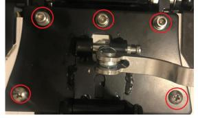
3. Tighten 3x Allen screws, fasten 2x Phillips screws under the turn signal with nuts. screw on the bottom.
