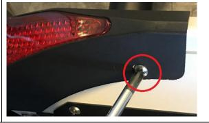
5. Squeeze the pin on the side of the holder, lift the seat and secure with a pin and a quick release lever.
