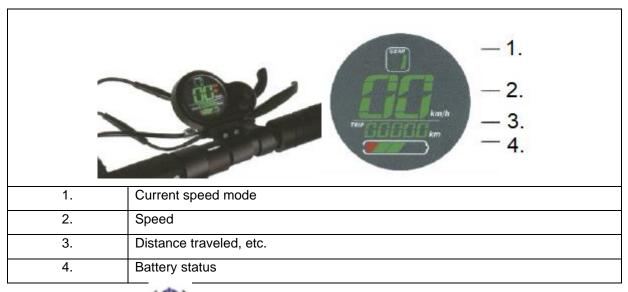
Hold the power button for 3 seconds to turn on. The LCD display enters standby mode.
