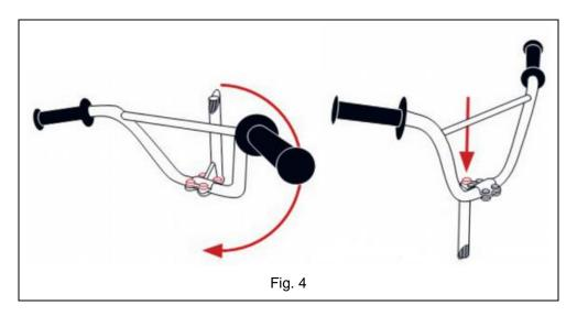
6. Insert the handlebar rod into the handlebar tube (Fig. 5). Adjust the handlebar height to the rider's needs. The maximum extension height is marked on the handlebar rod. Make sure the axis of the handlebars is parallel to the axis of the front wheel and properly tighten the screw (Fig. 4).
