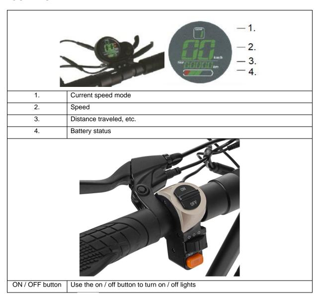
Hold the power button for 3 seconds to turn on. The LCD display enters standby mode.
