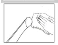
After use, hold the switch to turn it off and clean the head with a dry towel or napkin.
