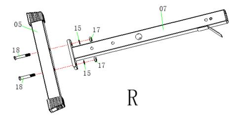
**Step 6**Attach the holders (6 and 7) to the main frame (1).
