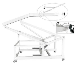
Attach bolt A7 to the front of the frame H. With this bolt you can adjust the vertical position of the board.
