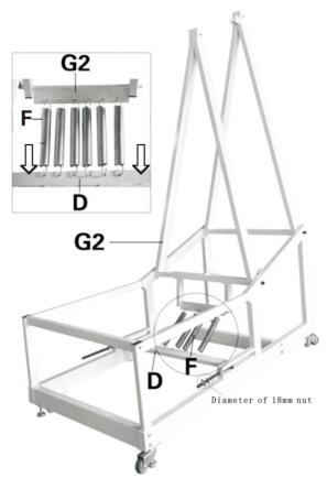
Pull the frame G2 as far back as possible and secure it to the frame C2 with a strong rope or twine. Be careful, sudden release can cause serious injury or death.
