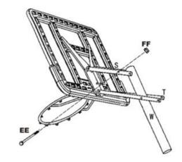
**Step 10**Attach big springs R to the board holder CC and to the bolt EE.
