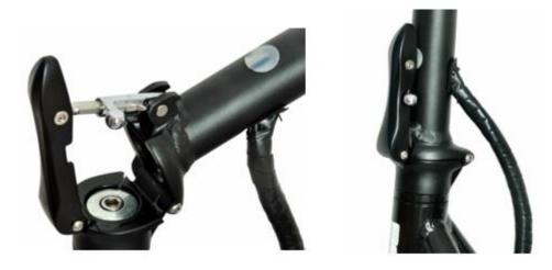
3. With quickrelease lever in the middle of the handles adjust the handles.
