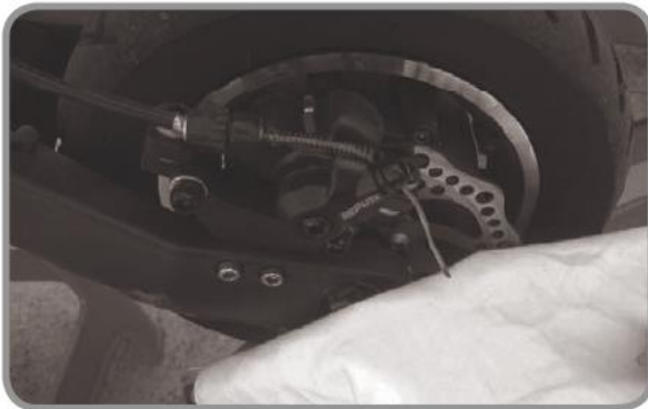
3. Clean the pads.
