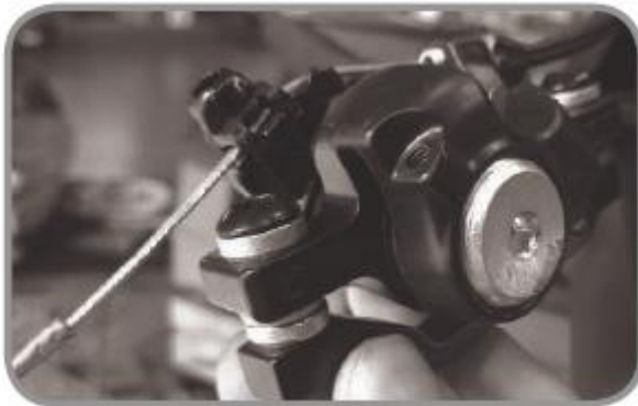
3. The bolt in the picture holds the pads, after replacement you must tighten them again
