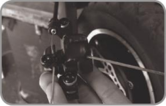
2. The brake caliper is separated
