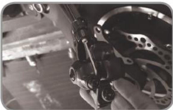
2. The brake caliper is separated
