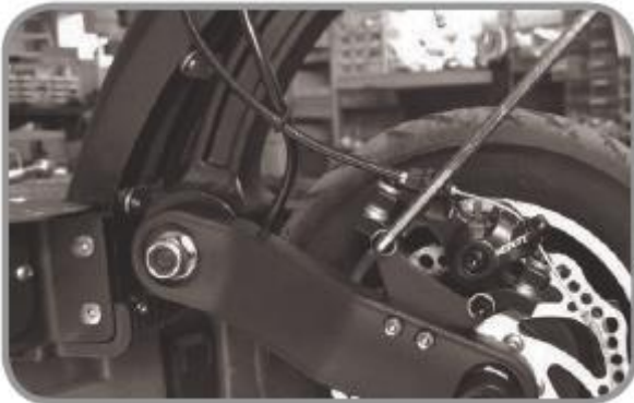
1. Loosen the bolt with a 5 mm Allen key
