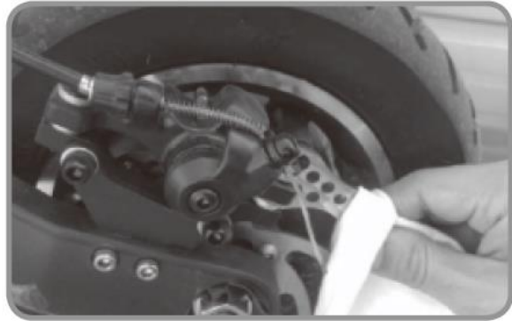
2. Clean the area where the disc and pads touches with a cloth.
