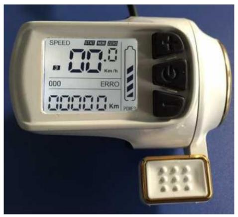
To turn on press  $\bullet$  button. After turning on press  $\bullet$  button to change displayed data: ODO (total distance), TRIP (current distance), RM, TM and error (chyby).
