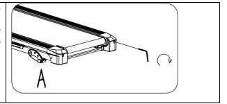
If the running belt (20) drifts to the left, turn the adjusting bolt on the left side ¼ of a turn clockwise, then turn the right adjustment bolt ¼ turn counter-clockwise. If the belt does not move, repeat this step until it centers. Refer to image B.
