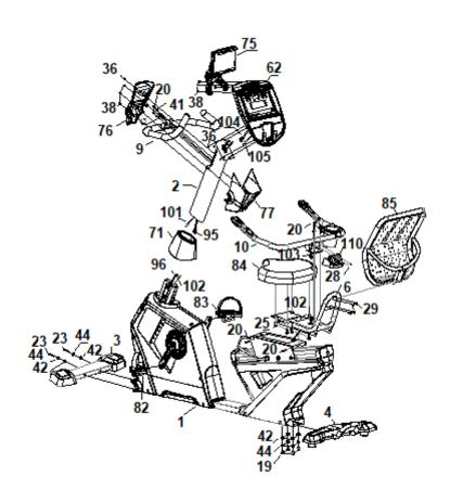
Attach the front stabilizer (3) to the main frame (1) using a flat washer (42), spring washer (44) and bolt (23).
