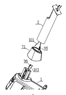
Connect the communication cables (95, 104) to the handle pulse cables (101, 105).
