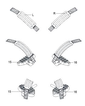
Remove the nuts (30 and 22), the metal bushes (28 and 29) from the right and left pedals (15 and 16). Insert the left pedal (15) into the bushing (28), the connection rod (10), the bushing (29) and the left crank (9). Then screw the nut (30) counterclockwise. Repeat for the right pedal (16), screwing the nut clockwise.
