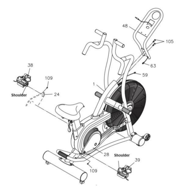
Insert two AA batteries into the console (85). Batteries are not included. Connect the connecting cable (63) to the console (85). Secure the console (85) in the console bracket (48) with the screw (106).
