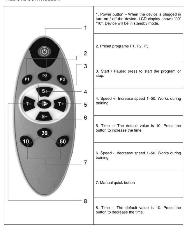
The controller has a range of 2.5 m.
