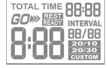
When you reach the last REST interval segment, the console will sound a short alarm and the workout will soon end.
