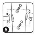
Secure the handlebars with 4 bolts M6x20 and spring washers.
