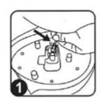
Connect the signal cable with the base.
