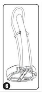
Fix the handlebars to the base with 2 bolts M10x30 and spring washers.
