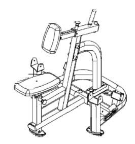
Above shows STEP 3 assembled and completed.
