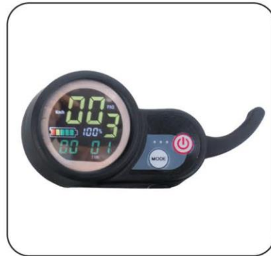
Accelerator / Switch Button/ Battery Indicator
