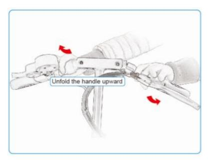
**NOTE**: Before each use make sure, that the safety switch is inserted all the way into the central folding mechanism. Otherwise you risk injury of yourself or mechanism breakage.
